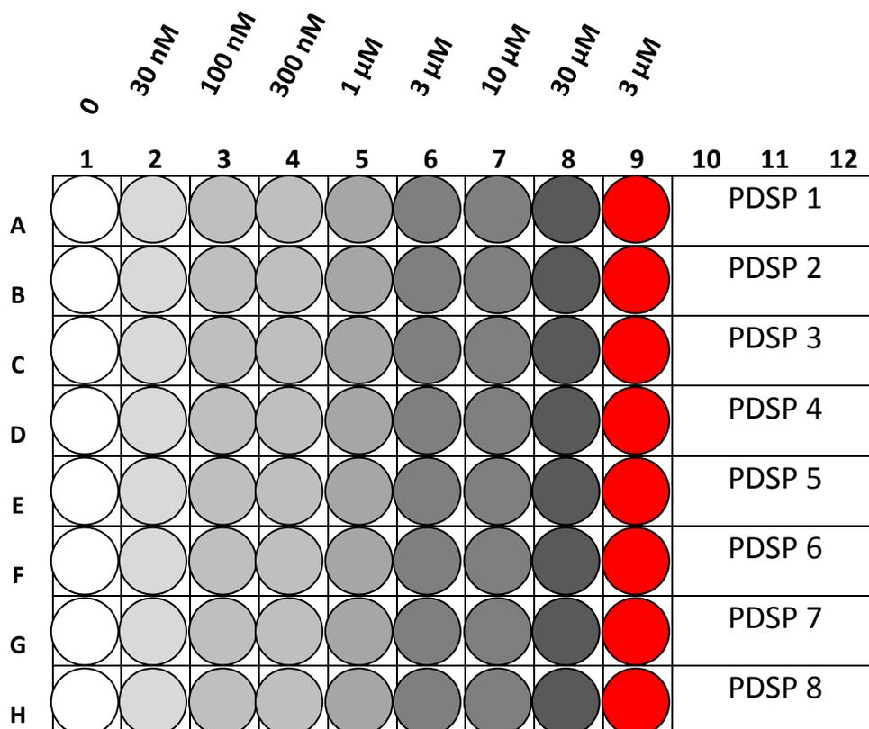
**Figure 55.** A typical APPC drug plate map (minimum of 360  $\mu$ l per well). Each drug has eight serial dilutions 0.5 log units apart as indicated in the plate map, starting with a buffer control on the left and ending at 30  $\mu$ M, followed by a positive control (**red**) on the right, usually Cisapride at 3  $\mu$ M.
